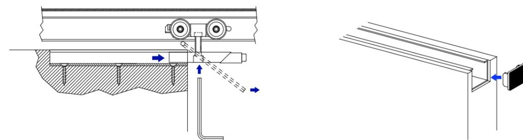
INTRODUIRE LES CHARIOTS (N) ET LA BUTEE D'ARRET (P) DANS LE LOGEMENT RESERVE. ACCROCHER LE VANTAIL AU CHARIOT AVANT, POUSSER LA PORTE A L'INTERIEUR DU MONTANT DE BUTEE. INSERER L'ETRIER ARRIERE ET REGLER LE COULISEMENT.
