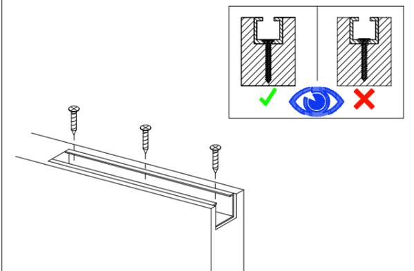
FIXER LE RAIL EN ALUMINIUM A LA PORTE AVEC LES VIS 4X30 FOURNIES. VERIFIER QUE LES VIS N'EMPECHENT PAS LE PASSAGE DE L'ETRIER.
